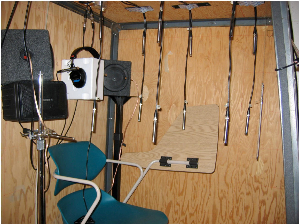
Figure 5.8 Microphones used to measure the performance of the ANC system.
