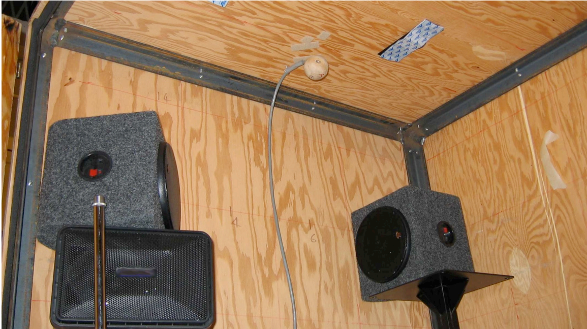
Figure 5.6 Satellite control speakers and ED error sensor placement.
